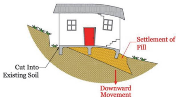
Figure 1-34. Settlement of fill resulting in cracks in the exterior wall finish.
